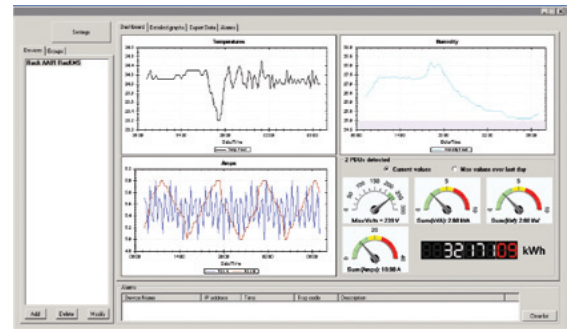
The low clutter dashboard shows all power and environmental data as trend lines for selected devices over the last 24 hours.
